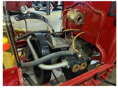
This 1907 Maxwell has a 127 cubic inch, horizontally-opposed two-cylinder water-cooled engine (with mechanically operated inlet valves) with a honeycomb radiator with thermosiphon cooling. Generating about 14 horsepower this vehicle would have produced a maximum top speed of 20 miles per hour. The transmission is hand-lever-operated planetary gearset with two forward speeds and one reverse.
