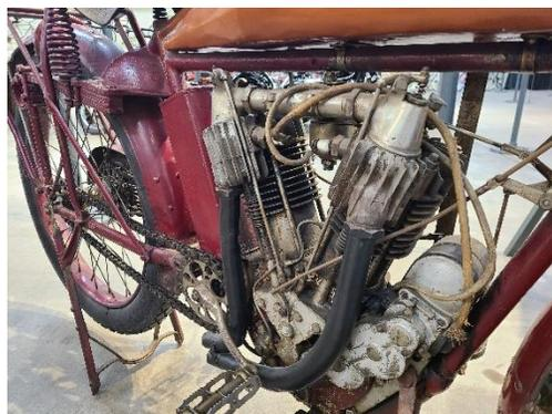
From a single F-head (inlet over exhaust) engine, by 1913 the Twin had an OHV 4-valves-per-cylinder, F-head design. Displacing about 61 cubic inches the 1913 had a bore and stroke of 3.25” x 3.67” and generated about 8 horsepower, for a top speed of about 50 miles per hour.
