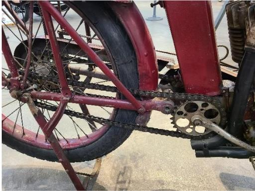
Another standout feature of this bike is the front and rear leaf-spring suspension. The first bike with front and rear suspension, it's possible the "cradle spring frame" was too bouncy since no form of damper was used with the leaf springs. The design lasted a few years, before being changed back to a rigid frame until the introduction of the plunger design in the 1940s.
