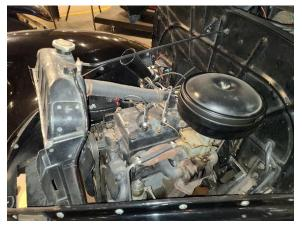
The 134.2 cubic inch engine is an inline L-head 4-cylinder, with a one-barrel Tillotson carburetor, providing about 48 horsepower. Despite the lower horsepower, the smaller-bodied Willys models of this time were still known for producing decent speeds with good fuel economy. Their light-bodies also made them popular with hot-rodders of the era. The transmission is a 3-speed floor-shift manual. This model came equipped with four-
