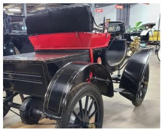
All Curved Dash Oldsmobiles are righthand drive with a steering tiller. A crank handle was permanently fixed to the engine and extended out the side of the body to allow the driver to start the car while seated.
