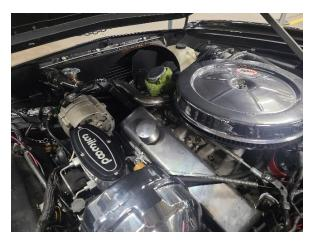
Highly modified mechanically from stock, the engine on this 1968 Avanti II is a 383 cu.in., 450 hp, GM Corvette V8 with an Edelbrock 750CFM Carburetor. A 6-speed Tremec T-56 Manual transmission, Moser one-piece axles and Auburn Gear Posi-Traction differential transfer that power to the road. With an estimated top speed
