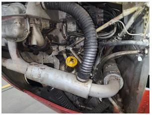
The Fornaire F-1 featured the Continental C-90-12F: a four-cylinder, horizontally opposed, air-cooled direct-drive engine of 201 cubic inches displacement. Used in many light aircraft built in the United States at the time, these popular engines produced between 90-100 horsepower. This four-stroke reciprocating engine is equipped with a fuel injection system and a redundant
