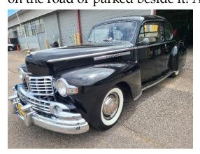
profile and chrome accents. The plush cloth interior made for a comfortable ride, and the fully appointed dash included an electric clock, radio and heater controls along with vehicle instrumentation. A unique Lincoln feature seen on this car are the pushbutton door handles, more streamlined than traditional handles. Electrically powered hydraulic windows are also seen on this vehicle.
